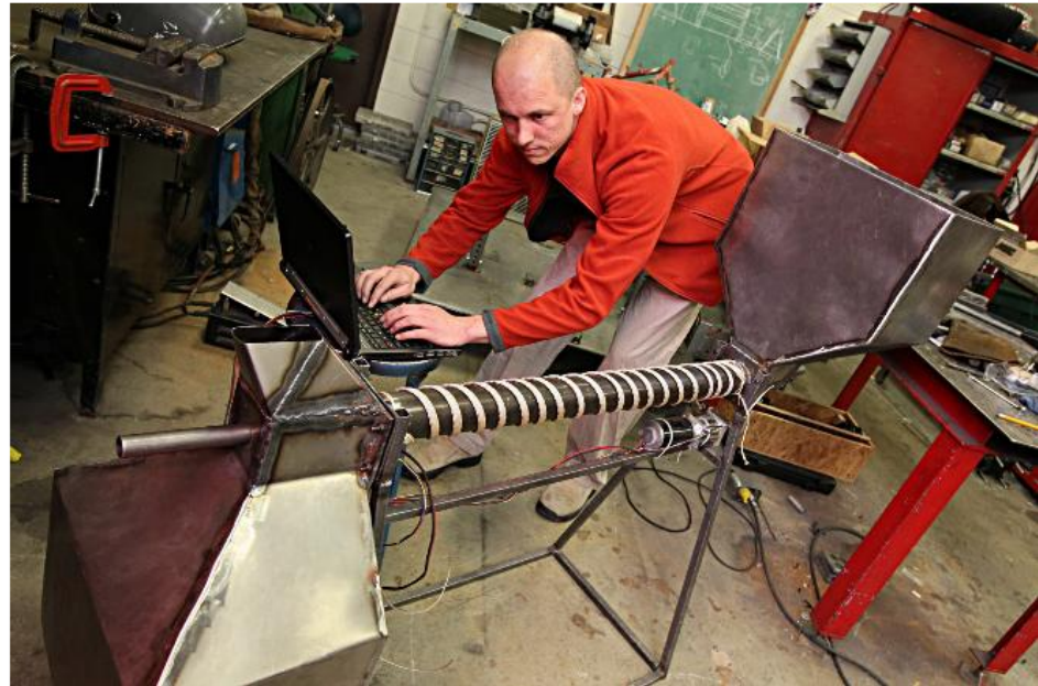
Michael Sears Navy veteran Jeremy Anderson, a mechanical engineering student at MSOE, works on his solar thermal biomass processor in one of the school's shops.
